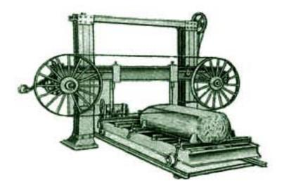
Trolley type wood working horizontal bandsaw machine having frame doubles steel channels and the long-carriage has steel structure with automatic movement of the carriage by gearing arrangement which provided accelerated return motion complete with suitable electric motor phase 440 volts, motor pulley, V belt, starter, suitable trolley and railings.
