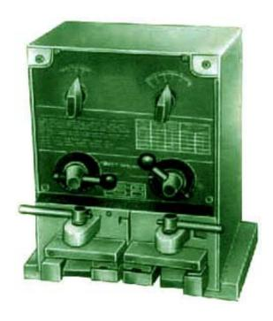
Indian make Bandsaw Butt Welding Machine model suitable equipped with welding and anneating attachment and suitable control switches.
