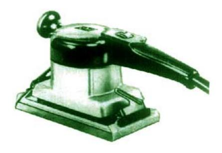
Portable orbital Sander used for sanding and polishing veneers, wood sheet metal primers of filters, to remove oil paint laquer, wall paper or rust equipped with special A.C. motor having shock proof insulation against 1500 volts, having sanding stroke 5 mm, sanding pad size 115 x 225 mm (1/2 sheet) motor watts 250 suitable for operation on AC 220 volts, single phase 50 cycles, 300 RPM electric supply, approx. weight 3.91 Kgs.
