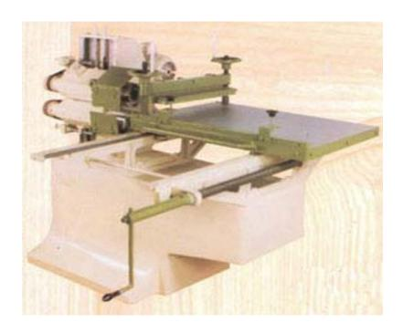
Motorised tenoning machine specially designed to make accurate and true tenons, double of single as required. The tenon heads are easily adjustable having max. length of tenons at one stroke 5" top or bottom tenon head will rise above table 4" dia. of tenon spindle 1.1/4" size of table 35" x 12.1/2" max. depth to cut 1.1/2", complete with 5 HP, AC 440/3/50 electric motor and starter.
