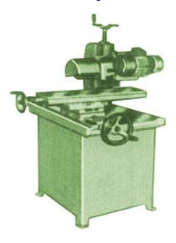
Motorised Wood Working milling machine with adjustable & tilting work head for milling straight and cross cutting of wooden planks such as for casing, capping, grooving tennonning, etc., equipped with 3 jaws self centering true chuck for holding cutters, moulding block and circular saw cutting attachment having table working surface 23" x 8" cross travel 12" vertical travel 24" spindle speed 3500 RPM complete with 2 HP AC 440/3/50 motor and starter.
