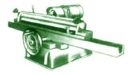
Planning Knife Grinder Sharpening Machine Model suitable for grinding, planning Knives and various types of blades, equipped with rack and pinion drive longitudinal slide for quick and faster grinder AC 440/3/50 electric motor - HP mounted on swivel graduated base, rotary "On" "Off" switch, cup type grinding wheel and wheel guard.
