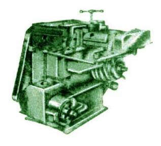
Best quality Indian Make (5 cuttery) heavy duty auto feed with 4 speed gear box complete with electric motor, motor pulley, V belt starter having the following specifications.
