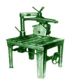
Best quality Indian Make Ribsaw machine complete with electric motor 2HP 3 phase, 2800 RPM 12" circular saw with saw guard motor pulley, V belt push button starter having the following specification.
