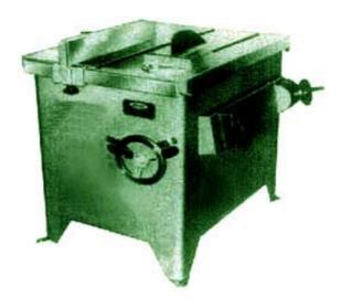
Heavy duty Fixed Table Circular Saw machine provided with tilting blade can be tilt upto 45° to cut wood in taper shapes provided with suitable electric motor 3 phase, 440 volts motor pulley, V belt and push button starter.
