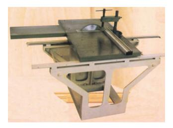
Motorised heavy circular saw machine provided with table has a rise and fall movement adjustment tilts upto 45° complete with suitable motor 3 phase, 440 volts motor pulley, V belt starter saw guard rip fence and one saw blade.
