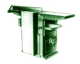
Heavy duty Cast Iron body floor model combined thickness and jointer (Surface planner) for planning of wooden stock provided with thickness planner with auto feed arrangement for feeding to wooden stock and surface planner with long surfacing table, cutter block with 4 nos. planning knives is provided for palining of woods complete with suitable electric motor 3 phase, 440 volts, motor pulley, vbelt and push button starter.
