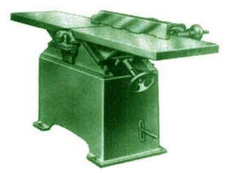
Heavy duty Cast Iron body motorised Surface cum Jointer planner suitable for planning of woods fitted with cutter block with 3 nos. planning knives complete with suitable electric motor 3 phase, 440 volts, motor pulley, vbelt and starter.
