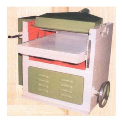
Heavy duty Cast Iron body thickness planner for planning of wooden stock provided with grooved roller on in-feeds side and plain roller on other side for automatic feeding of wooden stock with pressure adjustment vice, cutter block having 3 nos. of planning knives is provided with ball bearing, speed of cutter block is recommended approximately 4500 RPM, machine is supplied with suitable electric motor 3 phase, 440 volts, motor pulley, vbelt and push button starter.
