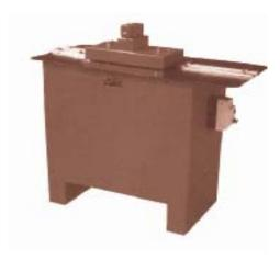
Principally used for joining sheet metal at right angles on straight runs, the machine comes complete with Pittsburgh rolls. Auxiliary shafts are fitted as standard, onto which double seam rolls can be fixed, When the flanging attachment is used with the machine (as illustrated) this makes possible the forming of round bends.
