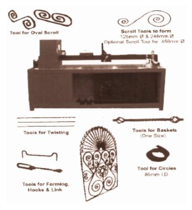
Wrought Iron working machine is very useful to make design in windows and doors from metal strips and bars and also in other bending works
