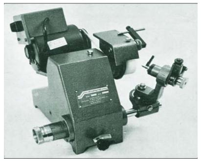
Scriptograf Cutter Grinder Model SG/CG-1 with Motor, Tool Head with Indexing device, collet 3.15MM OD Collet 6.35MM Dia. Nylon Belt, Diamond Dresser, A1. Oxide & Silicon Carbide Grinding Wheel, Diamond Grinding wheel & Instruction manual
