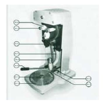
Scriptograf Inside Ring Engraver complete with Diamond Point and Brass Template A to Z along with 0 to 9 Digits
