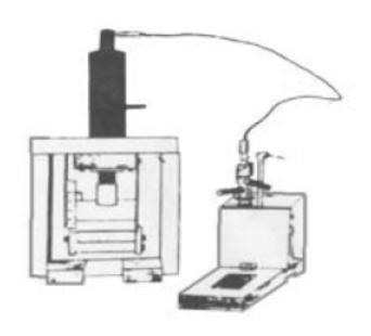
Vertical hydraulic hand operated bus bar bending machine ideally suitable for bend-ing copper, alluminium and mild steel bars.
