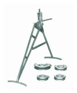
Model GCP Hand operand thin walled (ERW) furniture or conduit pipe bending machine is suitable for bending pipes from 1/2" to 1.1/4" die. without filling or heating etc.. with centre formers and outer formers. Capacity: 1/2" to 1.1/4" dia. Size of standard formers supplied 1/2", 5/8" 3/4", 1"and 1.1/4" Approx. weight: 40 kgs.
