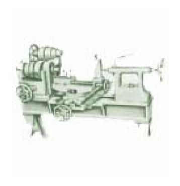
Motorised floor model spinning lathe with taper roller bearings, for spinning flatcans, light metal turning, smoothening, trimming, beading, curling, complete with beading & triming attachment, motorisation attachment motor pulley, vee belt suitable H.P. A.C. 440/3/50 electric motor and switch
