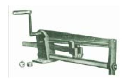
hand operated grooving or side seaming machines, for closing side seams on round or irregular shaped bodies with detachable mandrel having full length groove for inside seams complete with a set of grooved two wheels for outside seams and one plain wheel for inside seam.
