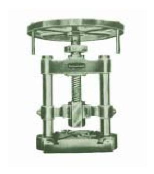
Heavy duty double pillar type hand driven screw presses specifically designed to draw numerous sheet metal articles, utensil hollow-wares, containers, bottle tube caps etc. and also useful for embossing, punching, numbering pressing etc. complete with fly wheel and handle.
