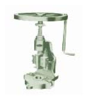
Hand operated fly presses with two adjustable vee guides provided with oil grooves for constant lubrication complete with 2 catch dogs with bolts and nuts. Fly wheel or handle with ball weights as desired (fly presses No. 0.1 and 2 are supply with fly handle with one ball weight only or wheel as desired).
