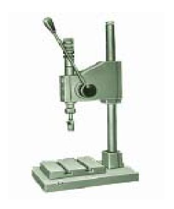
Impact press with adjustable striking load, the adjustable arm and wide throat permit using the press in various industries like electrical control equipment, switch gear, domestic appliances, radios, telephones, materials equipment, cycles, office equipment, ammunition, automobile ancillaries etc.
