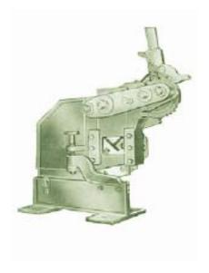
Heavy duty geared shearing machines equipped with rack and pinion arrangement with a ratchet gearing mechanism which reduces the physical effort appreciable, fitted with a swivel type down holder in the front and a feed guide-cum-down-holder for sections in the rear, supplied with standard set of blades for cutting sheets, flats, angles, tees, round, square bars and a long operating handle having following specifications:
