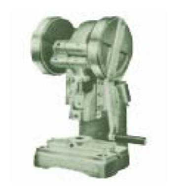
Hand operated toggle action bench press ideally suitable for blanking, piercing, rivetting, bending or punching, T-slotted table is provided with tool bolster for circular type die, and setting plug for alignment. The ram is adjustable for tool height.
