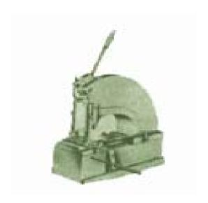
Hand operated single station multipurpose punch press which perforates holes of various sizes and shapes upto 4" dia. hole in 16 swg. mild steel sheet rapidly and efficiently. with adjustable side and backgauges punchholder for punches with 1/2" dia. shank die holding, handle for operator convenience
