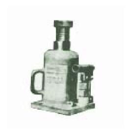
All steel welded construction 25% overload tested hydraulic jacks with integral pump having 150 mm hydraulic lift available in two types (1) Plain Ram (2) Screw Ram with safety lock nut
