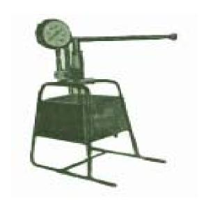
Hydraulic test pump designed for testing pressure cap. of different materials like drums, valve, boilers, barrels, tanks for pressure vessels and cylinders complete with stand, pressure gauge, check valve and outlet valve with water tank having following specification.
