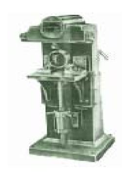
Hand operated stamping machine suitable for stamping on any metal, square, flat or round materials, stamping capacity 5/16" to 4.1/2" dia, having size of square table 9" x 7", complete with handle, Approx. weight 150 kgs.
