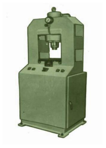
Hydraulic Coining press ideally suitable to make impression on gold and silver coins. The machine is equipped with 5 H.P Flange type 1440 Rpm. Electric Motor,
