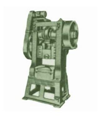
Heavy duty double column press with adjustable stroke suitable for punching embossing, deep drawing work, body rigid casted double column mounted on heavy cast iron legs reinforced with tie bars equipped with balancing fly wheel, drive gears required A.C. 400/3/50 electric motor, starter and foot operated clutch:
