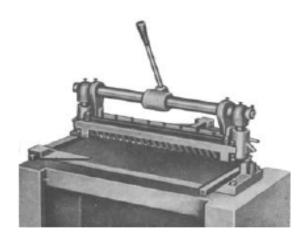
Hand operated bench type shearing machines suitable for production operations in all shearable materials including Plastic, fibre, mica, rubber, leather, alluminium, copper, cobalt steel, chrome, molybednium, lead, brass & stainless steel,
