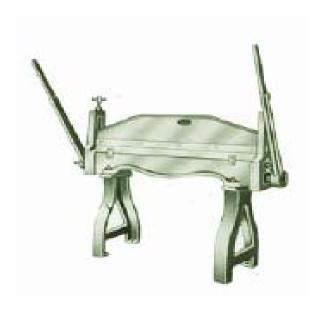
Heavy duty hand operated trunk folding machines specially suitable to form heavy and large right angle and curved folds on the sides of the trunks and also suitable for folding the sides of trays and various other similar articles with help of suitable dies, operation through the bed by eccentric shaft raising and lowering the top beam, top beam has adjustment for height, complete with one M.S. bending die for 90 deg. (square) bends, a set of gauges and bench mounting stand.
