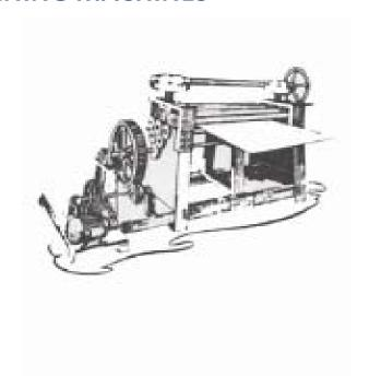
Motorised geared heavy duty nine rolls sheet straightening machine equipped with nine rolls running in bushes suitable for straightening plates upto 1.6 mm (16 swg) sheets complete with 5 H.P. AC 440/3/50 electric motor, switch and belt maximum width of sheet admitted 910 mm.
