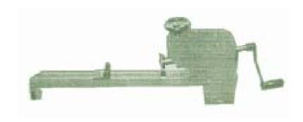
Gasket Cutter produces clean, accurate cuts in most Jointing Materials up to 6.4 mm (1/4") thick approximately. This equipment is strongly recommended for producing Gaskets from compressed Asbestos Fiber Sheet. Its simple adjustment and operation make it easy to cut Joints effectively and professionally, permitting there-use of the off-cuts.
