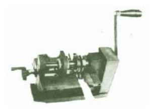
A) Hand operated Precision Strip cutting machine especially designed to obtain strips having a very extra breadth. It can cut the strips in various breadths with the adjustment of a micrometrical screw within any change of parts, equipped with four knives, two of them are sliding on the axis. The knives are interchangeable and can be re-sharpened, having capacity to cut maximum thickness of metal upto 0.7 mm, minimum width of cut 6 mm, maximum width of cut 40 mm.
