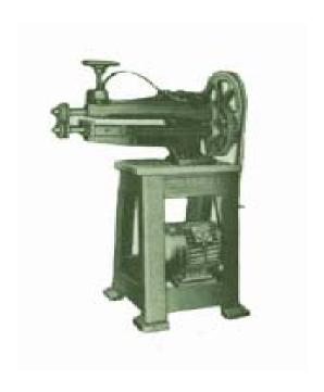
Model DSM-18 deep throat swaging machines are suitable for swaging, jennying, burrying, oggling, beading, closing and various other operations on drums, buckets and tin containers complete with one pair of swage rolls.
