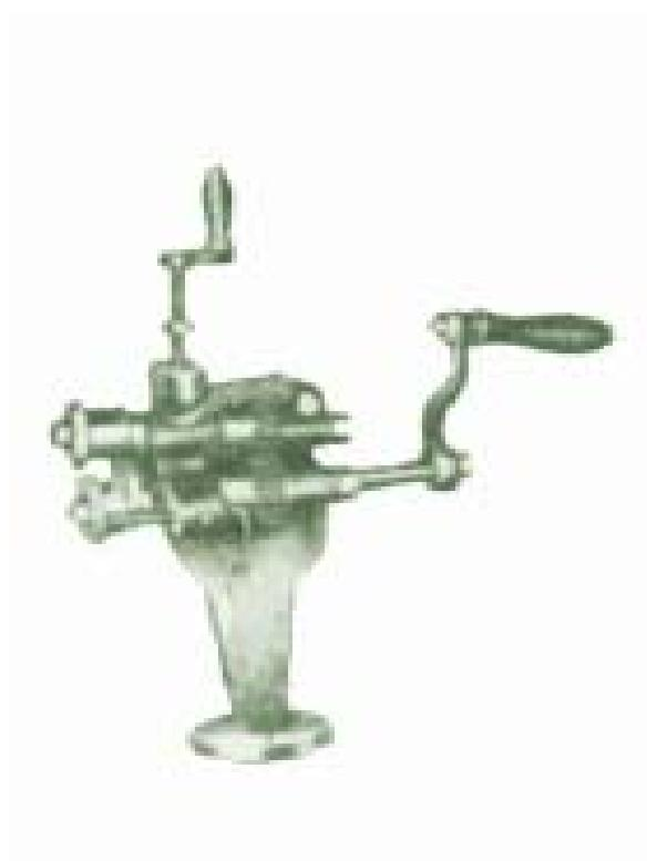
Hand operated jenny or burrying machine model JNI designed for edging, flanging or burrying the edge of all classes of tin plate work of any shapes, generally used for edging and flanging bottom and bodies to various angles previous to, panning or setting down, double seaming etc. provided with an adjustable gauge, one pair jenny rolls and mounting bench, dia of rolls 1.1/2" max. depth of gap to gauge 5" and handles work of thickness upto 22 swg. MS. complete with handle.
