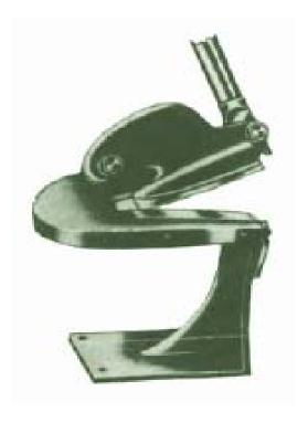
Hand operated Curve cutting shear for cutting various shapes, curves and making angle cuts, as well as straight cuts with a capacity to cut M.S. Sheets in unlimited length upto 3mm (1/8"), length of blade approx. 4"
